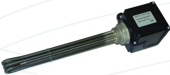
Immersion screw-in heaters are used for direct heating of water in stainless steel and enamelled tanks. It consists of 3 "U"- shaped tubular heating elements and a sensor protection tube, which are mounted in a screw head G 6/4". The Heater is with a plastic housing, in which a temperature control (30-75°) with a limiter (98°C) and indicator lamp is provided. Tubular heaters and screw head entirely of stainless steel.
